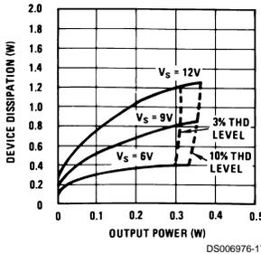
Device Dissipation vs Output Power — 8Ω Load
