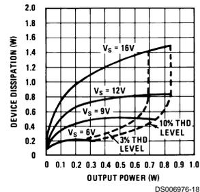
Device Dissipation vs Output Power — 16Ω Load
