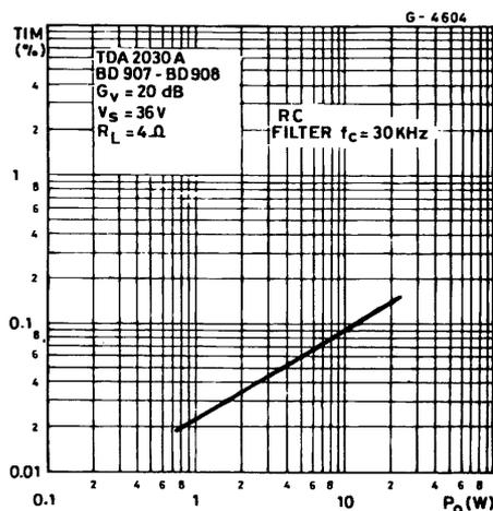
The diagram of Figure 26 originated by SGS-THOMSON can be used to find the Slew-Rate (SR) required for a given output power or voltage and a TIM design target.
