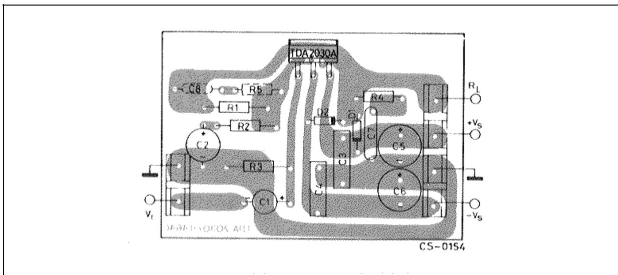
**Figure 16 :** Bridge Amplifier with Split Power Supply ( $P_O = 34W$ ,  $V_S = \pm 16V$ )
